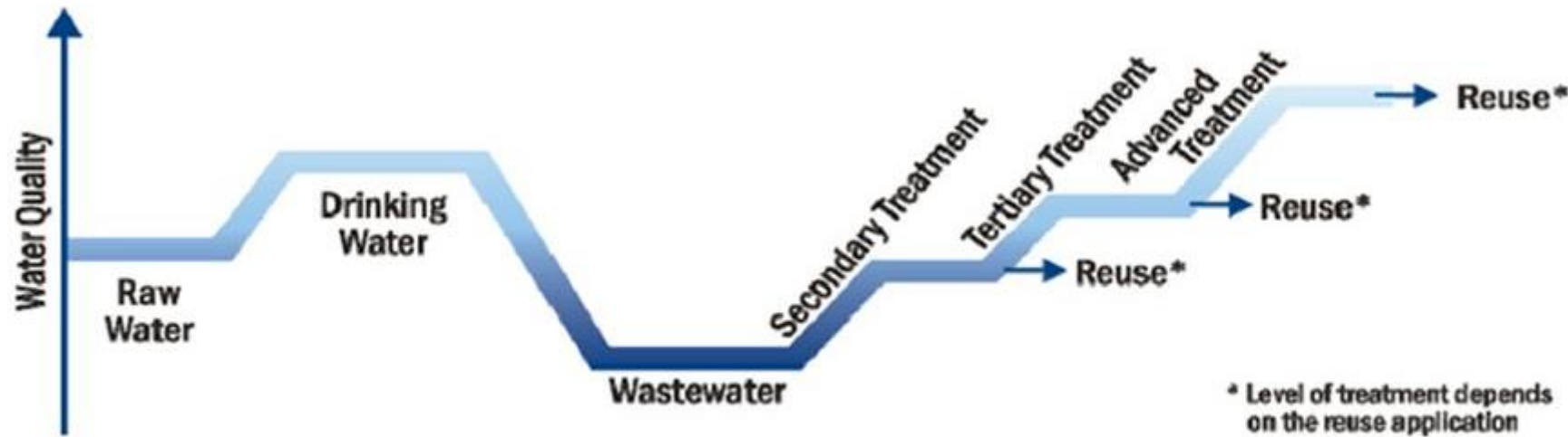
Figure 1-3 Treatment technologies are available to achieve any desired level of water quality
