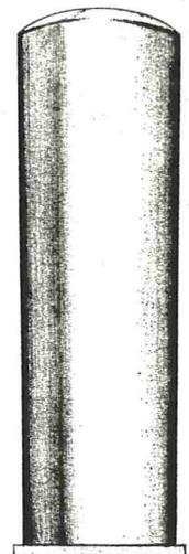
The typical Taper-Wall milk storage tank illustrated above has a diameter of 12 feet and a height of 50 feet. The product contact surface is stainless steel with a No. 4 finish.
