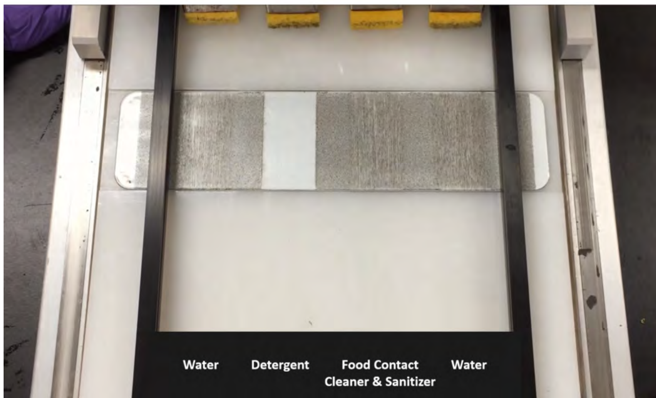
FIGURE 2. Kitchen-style baked-on greasy soil on a surface cleaned with a scrub tester. Cleaning agents were water (control, far left and right columns), a commercially available heavy duty dish-cleaning agent (detergent, second from left), and a food-contact cleaning agent and sanitizer product diluted as per label use directions (third slot from left). Sponges containing a fixed amount of each cleaning agent under identical pressure (via fixed weights) stroke the soil-coated slab 10 times. Qualitative soil removal after 10 strokes is depicted. (Procter & Gamble Professional, 2023.)
