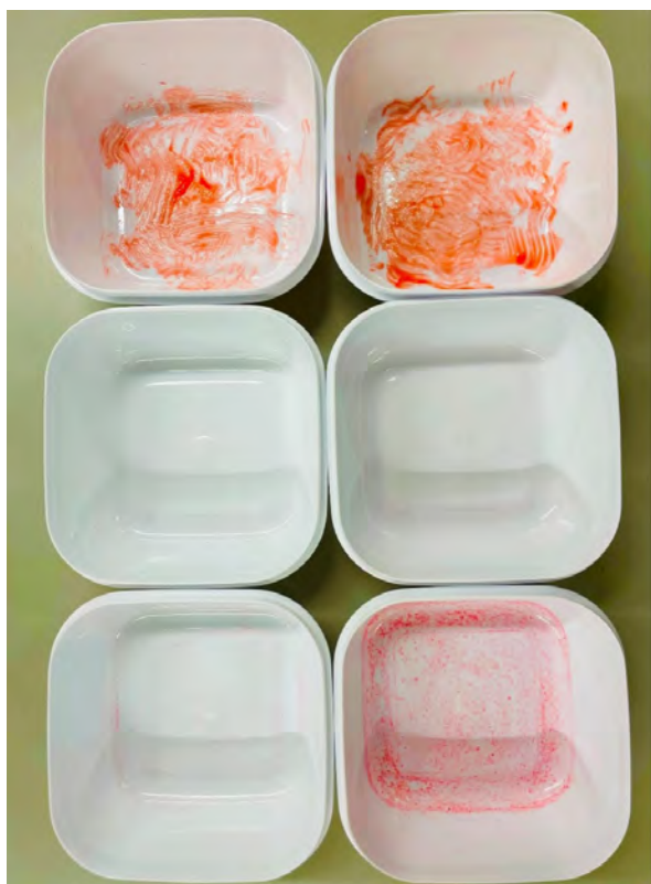
FIGURE 1. Cleaning performance difference between two commercially available cleaning agents. Two identical dishes (first row) contain greasy soil with grease-dissolving dye. Dishes were cleaned with commercially available cleaning agents A (second row, left) and B (second row, right) according to each cleaning agent label use directions. After applying additional grease-dissolving dye to the cleaned dishes, previously invisible and lingering residual grease is more apparent on the dish that had been cleaned with agent B (third row, right). Agent A was better for cleaning the greasy soil. (Procter & Gamble Professional, 2023.)
