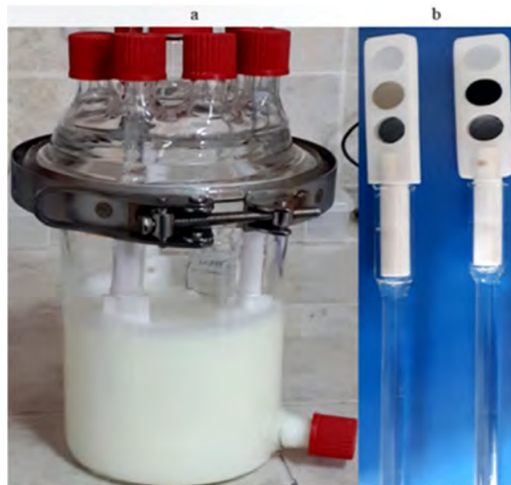
Figure 1. (a) The modified CDC reactor. (b) The holders placed with ideal abiotic surfaces.
