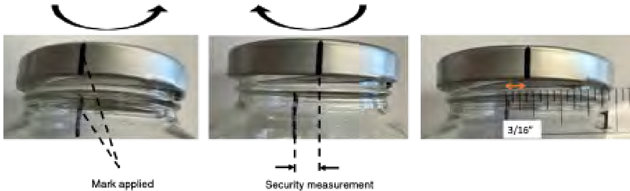
FIGURE 5. Security measurement for a glass jar with a metal lug closure.
