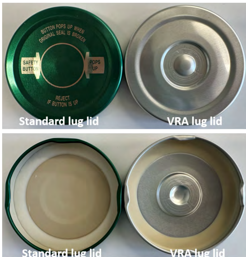
FIGURE 1. Face (top) and reverse (bottom) of standard lug and vacuum release aluminum (VRA) lug lids evaluated.
