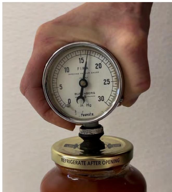
FIGURE 3. Vacuum measurement obtained by piercing the metal lid with a vacuum gauge.
