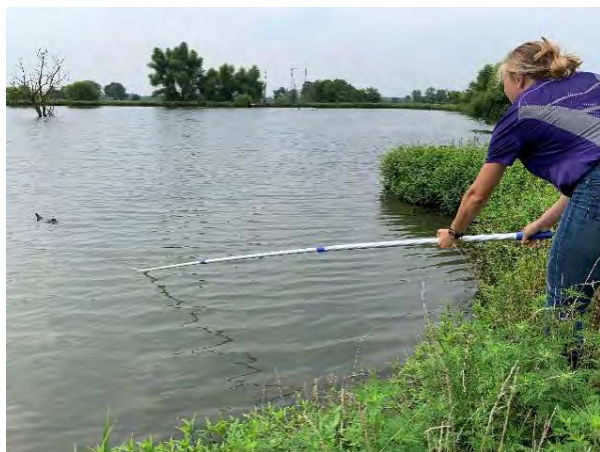
Figure 1. Depiction of method used to collect samples from surface water sources by using a collection bottle fixed to a long pole in a way that allowed the bottle to enter the water inverted just below the surface of the water, be rotated to collect the water sample, and turned upright to be removed from the water.
