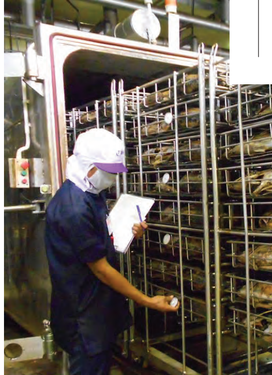
Tuna End Point Internal Product Temperatures (EPIPT) are measured upon discharge from the pre-cooker.
